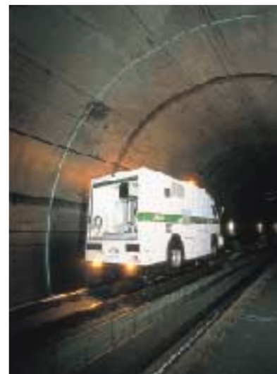
New Tunnel Inspection Car Replacing visual inspections, a new tunnel inspection car now examines tunnel interiors using sophisticated laser equipment. This raises both speed and accuracy of these inspections (see text).
